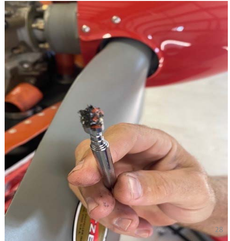
Metal Pieces from Oil Attracted to Magnet
