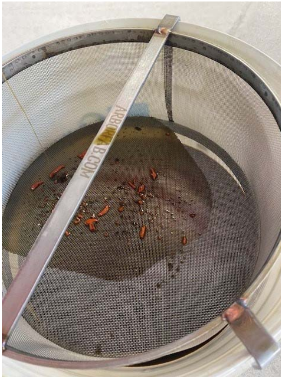
Metal and Elastomer Pieces in Oil Screen
