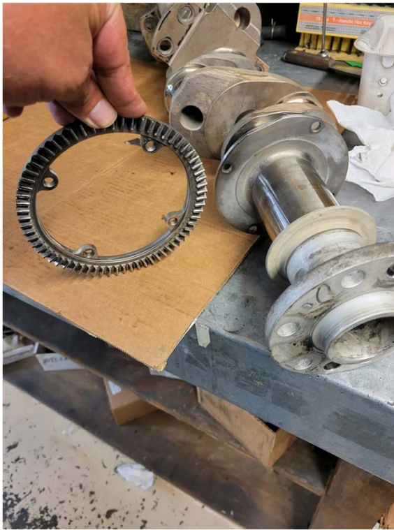
Face Gear Removed from Crankshaft
